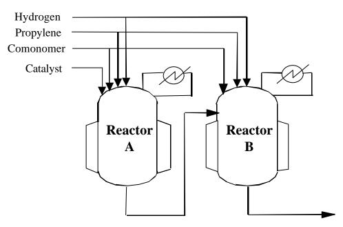
Figure 3. Continuous Liquid-Pool Process Flow
