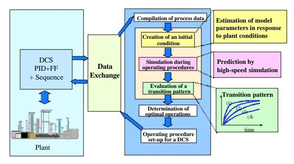
Figure 5. Determination of Optimal Operating Procedures and Integration with Control Systems
