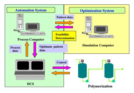
Figure 4. System Structure for Automatic Grade Transitions
