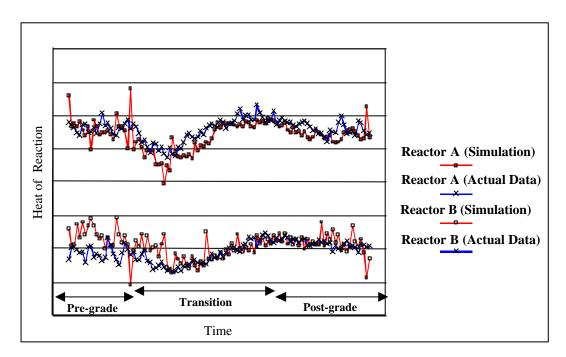
Figure 6. Heat of Reaction during a Grade Transition
